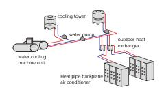
Schematic diagram of the air conditioner + heat
